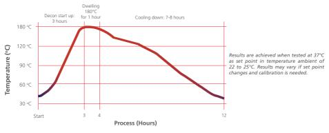
Figure 4. Graph of a full cycle sterilization process. Complete cycle lasts up to 12 hours.
