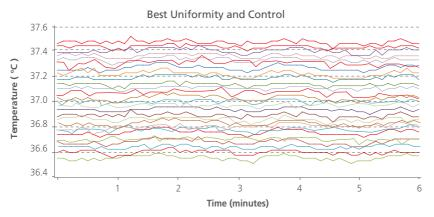
Figure 1. Different lines represent 27 sensors positioned inside the chamber. Esco CelCulture<sup>®</sup>  $CO_2$  incubator has uniformity variance of less than  $\pm$  0.5 which means all the samples are evenly heated.\*
